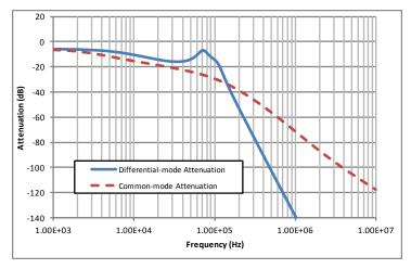
**Figure 1:** Typical Common Mode and Differential Mode Attenuation provided by the filter as a function of frequency. Source and load resistance are  $50\Omega$ .
